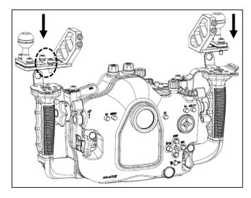
Take the two existing S.S. screws from mounting ball for the left bracket, and install the left & right bracket to the designated area.
