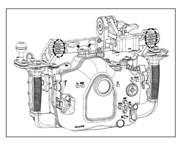
Install the adaptor to #17951 Mounting System by tightening the four S.S. screws as shown.
