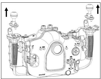
Unscrew the four S.S. screws, and remove the mounting balls from housing handles as shown.
