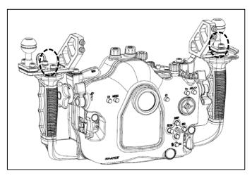
$\label{thm:continuous} \mbox{Tighten them with the four S.S. screws.}$
